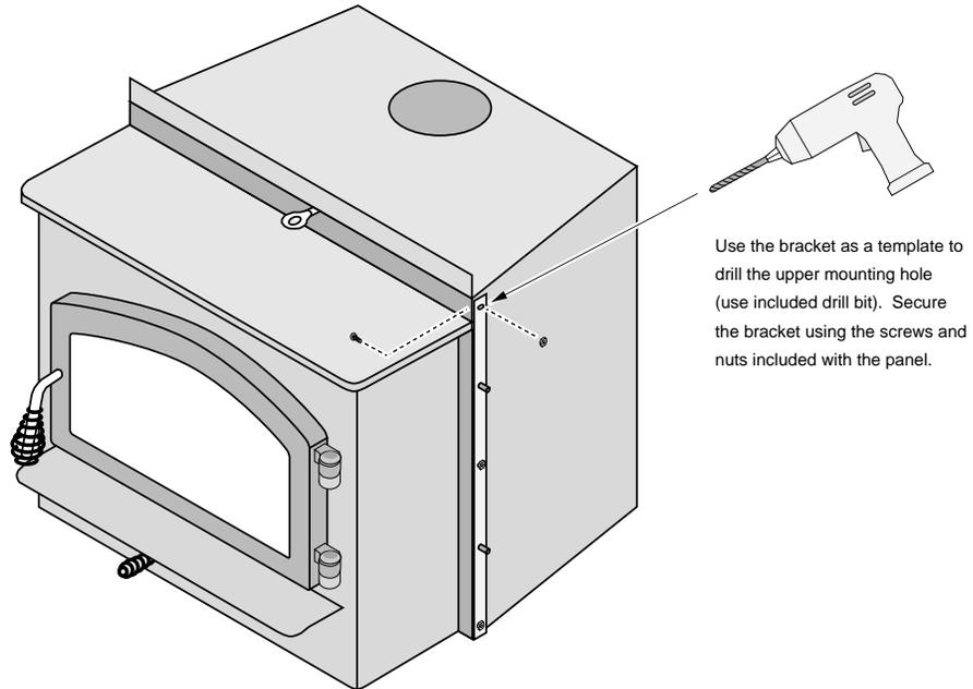
4. Place the insert into position (flue attached). Attach the surround panel as shown below.
