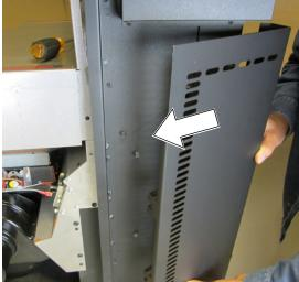
NOTE: When installing, make sure the tabs on the panel insert into the slots on the front of the insert
