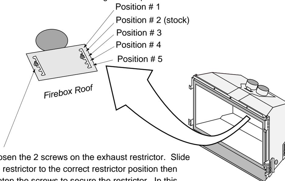
Loosen the 2 screws on the exhaust restrictor. Slide the restrictor to the correct restrictor position then tighten the screws to secure the restrictor. In this illustration, the restrictor in position 2.
