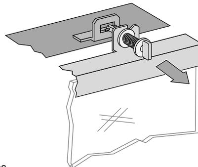
The latch will then disengage from the latch bracket.
