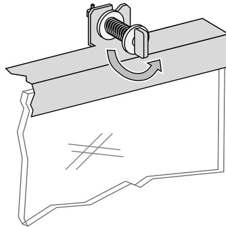
Once fully inserted, turn the latch until it is level.
