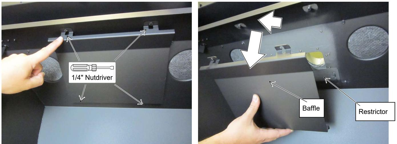
The restrictor is adjusted by loosening the two screws holding it in place. Slide the restrictor until the correct notch falls over the screws and re-tighten. Replace the baffle.
