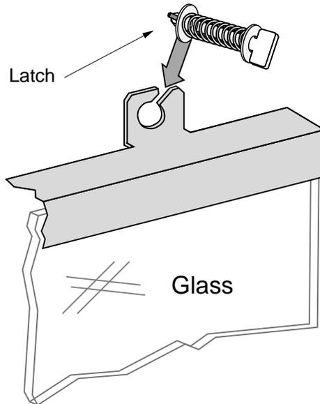
Hold the latch at an angle and insert it into the slot on the glass frame. Note how the washer fits in front of the flange on the glass frame. You will need to push slightly to get the latch to insert.
