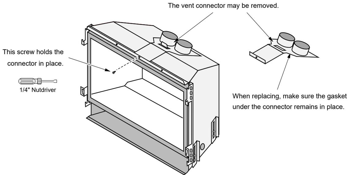
The vent connector slides back and disengages from the three tabs on top of the insert.
