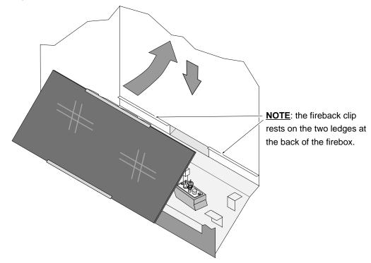
6 Install one of the side panels into the firebox as shown below. .
