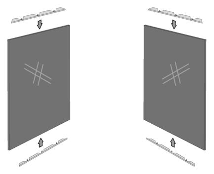
4 Prepare the rear panel for installation. Slide a spacer over the top and the bottom of the rear glass panel and secure the spacers in the same manner as the previous step.
