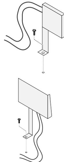
3. Attach the new light bracket to the insert as shown to the right.
