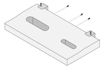
2. Attach the correct air deflector to the burner with the screws removed earlier. Note how the LP air deflector has a notch along the bottom.
