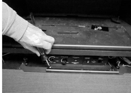
The switch bracket attaches to the Shadowbox face. Remove the two lower inside nuts (see photos below). Place the switch bracket over the studs and secure using the nuts removed earlier.
