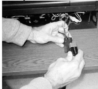
Remove the three nuts securing the LED bracket to the concealment cover (retain the nuts). Carefully place the LED bracket in front of the insert, making sure the wiring is not damaged.
