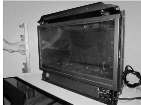
2. Remove the screw from the upper air deflector on the right side.
