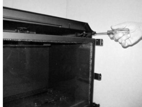
4. Attach the latch bracket to the left side using 3 of the included screws.
