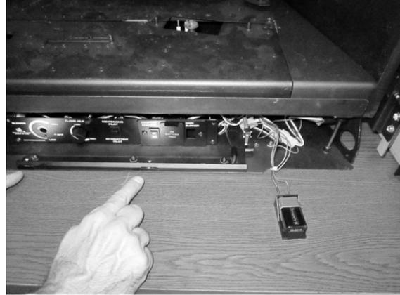
The last step is to verify the switch bracket properly contacts the micro switch on the insert:
