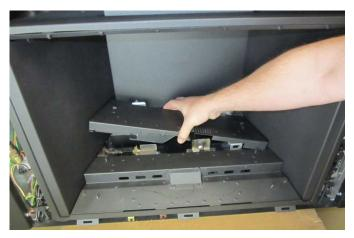
2. Remove the 3 screws from the back of the rear burner (1/4" nutdriver).
