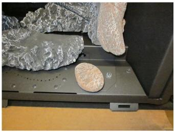
15. Place the right twig as shown below. The twig rests on the indent on the front ember chunk and the #4 stone.
