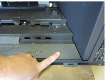
15. Secure the front-right log support to the stud using one of the included nuts (3/8" nutdriver).
