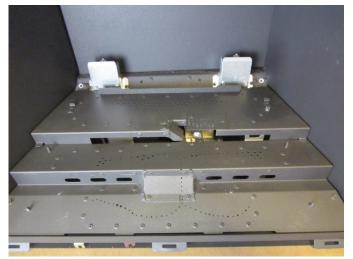
6. Position the rear log shelf so the two holes on the shelf fit over the two holes exposed in step 4 (rear leveling bolt cover plates).
