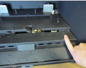
11. Secure the mid-right log support to the stud using one of the included nuts (3/8" nutdriver).
