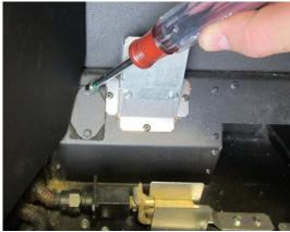
5. Replace the rear burner and secure with the screw removed earlier. Note how the two tabs on the rear burner fit over the front burner.
