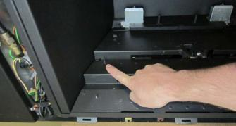
9. Secure the mid-left log support to the stud using one of the included nuts (3/8" nutdriver).
