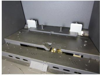
8. Place the mid-left log support over the stud on the left side mid-burner.
