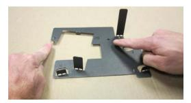
4. Attach the right stone grid to the burner as shown below. **NOTE:** When installed, the grid sits flat on the burner.
