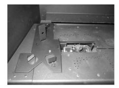
Place the rear stone grid on the burner as shown below.
