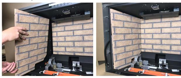
5. Replace the left fireback clip to secure the right fireback in place
