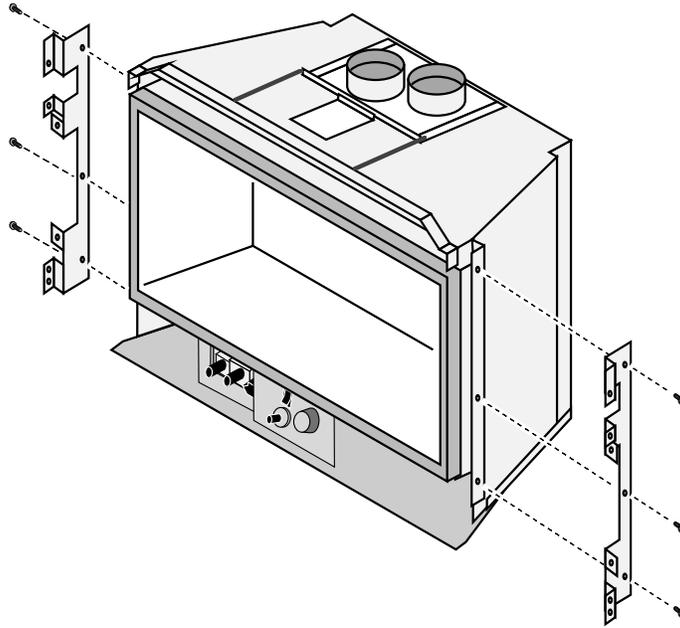
Attach the mounting brackets included with the backing plate.
