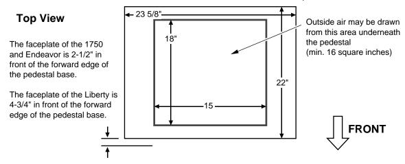
The Liberty wood stove can draw combustion air from the inlet near the air control. When using outside air you will need to install the included cover plate so all of the air is drawn from below. See the directions below.
