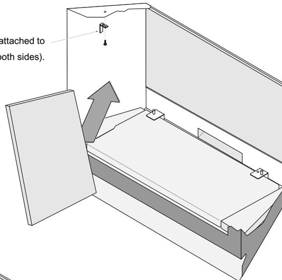
Hold the side firebacks at a slight angle and place them into position (both sides).
