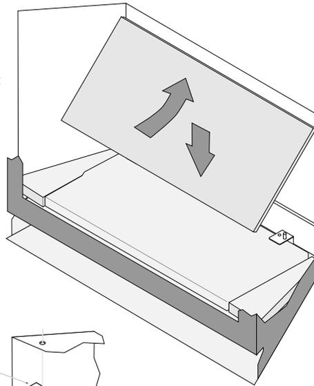
The fireback clip has a keyhole slot. It can be removed by loosening the screw and sliding the clip out.
