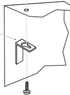
Remove this clip attached to the firebox ceiling (both sides).
