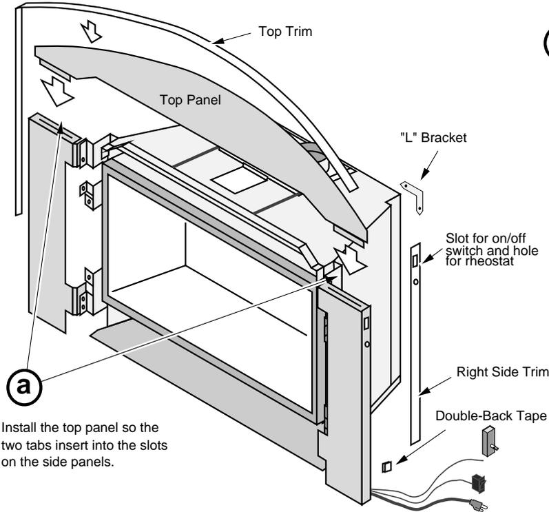
**b** Construct the panel trim. Insert one leg of each "L" bracket into the top and side trim piece as shown below. **NOTE:** The "L" bracket must be installed as shown - make sure the set screw may be tightened from behind (remove and re-install if necessary). Align the trim to form a precise corner, then tighten the two set screws with a small standard screwdriver. Slide the trim over the panels.
