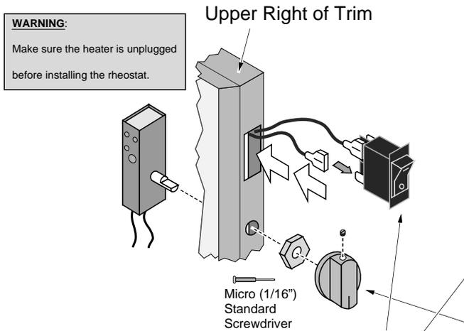
**a** Disconnect the red and brown wires leading to the on/off switch. Insert the wires through the rectangular mounting hole (on the surround panel or control panel) and attach to the on/off switch. The wires must attach to the top and bottom posts on either side of the switch -it does not matter which wire is on top. Press the switch into the rectangular hole until it locks into place.
