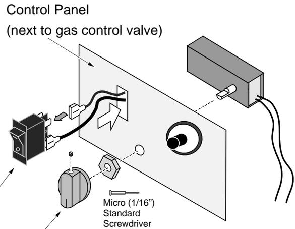
**b** Remove the knob and nut from the rheostat (the knob is held in place with a set screw). Insert the shaft on the rheostat through the circular hole (on the surround panel or control panel). Secure with the nut. Replace the knob.
