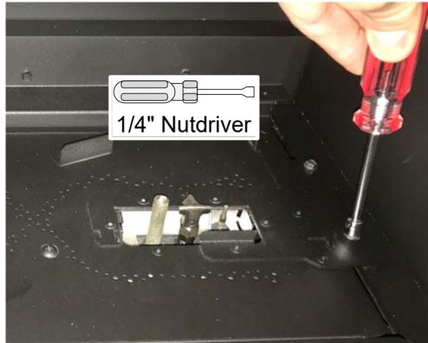
Remove the burner and place it aside.
