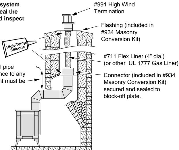
**\*CAUTION:** This vent configuration is not covered under the appliance safety standard (ANSI Z21.88 CSA 2.33) used in the safety certification of this appliance, however, this method has been tested by Travis Industries and it has been determined to be safe following the instructions above. Before installing the appliance using this method, contact the Authority Having Jurisdiction to determine if this installation is acceptable in your area.
