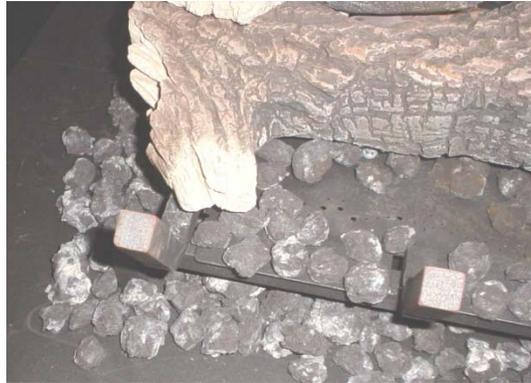
NOTE: When placing the embers, place one ember on both sides of the accent light deflectors (see illustration below). This helps block light from exiting the slot on the deflector and creating a line of light.
