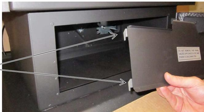
2. Remove the exhaust channel cover plate and gasket (a single wingnut holds it in place). When replaced, make sure the gasket on the cover plate seals the cover plate against the exhaust channel.
