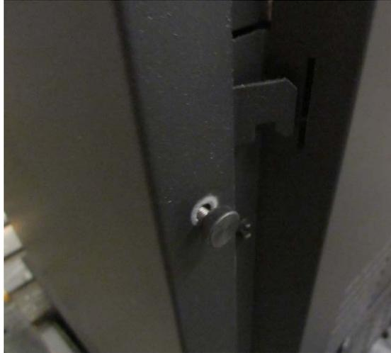
3. Slide the side panel back, tilt it outwards, and remove it from the stove. Note how the panel is held in place with three tabs on the back.
