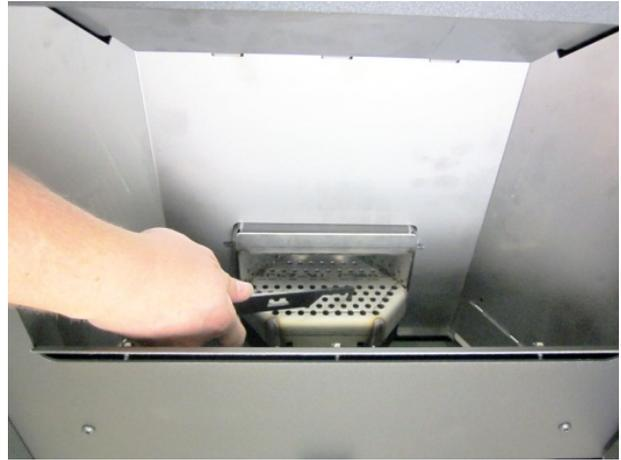
4. Brush away flyash around the burn platform using the brush included with the stove. The flyash will fall into the ashpan below.
