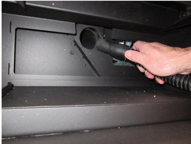
4. Clean the combustion blower with the bottle brush or vacuum.
