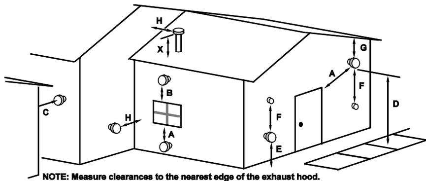
A Minimum 4' (1220mm) clearance below or beside any door or window that opens. (This clearance may be reduced to 18" if using outside air (see page 13) – we recommend the door or window be kept closed during operation.
