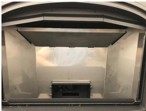
2. Lift the top center panel of the fireback up to release it from the notches on the lower panels. Lower one side and guide the panel out of the firebox.
