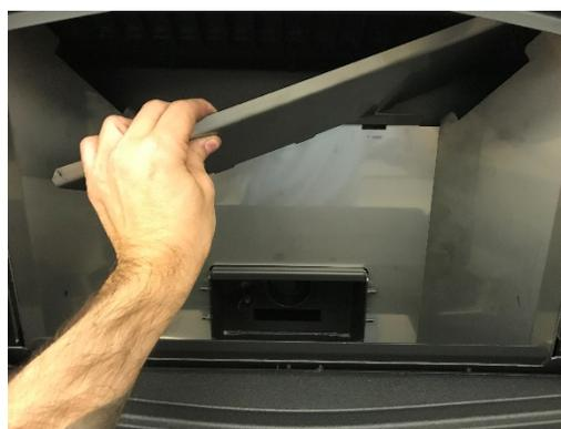
3. Lift up on one of the side panels to release the (2) tabs on the bottom of the panel from the notches in the firebox. Guide the bottom of the panel forward until it can be lowered into the ashpan area.
