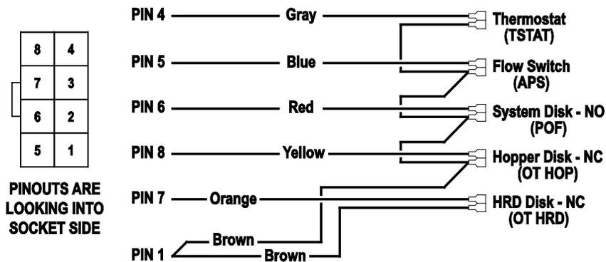
NOTE: text in parenthesis match power control board printed characters
