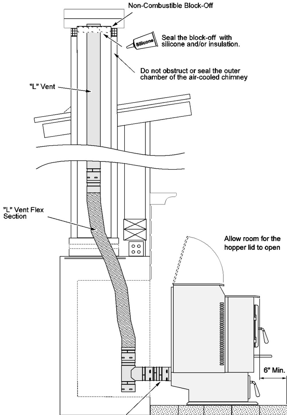
**NOTE:** you may need a short horizontal section here to clear the lintel and allow the hopper lid to open.
