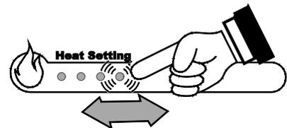
**TIP:** If the stove turns on and off repeatedly, you may wish to turn the heat output to a lower setting. This provides a more consistent heat output, eliminating the need for the thermostat to turn the heater on and off.
