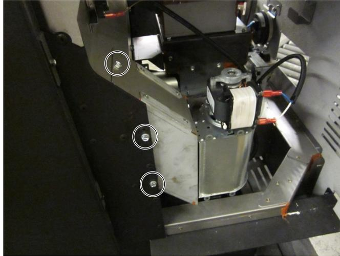
Disconnect the blower assembly (the wiring may remain in place during cleaning). Clean all dust and debris from the convection blower.
