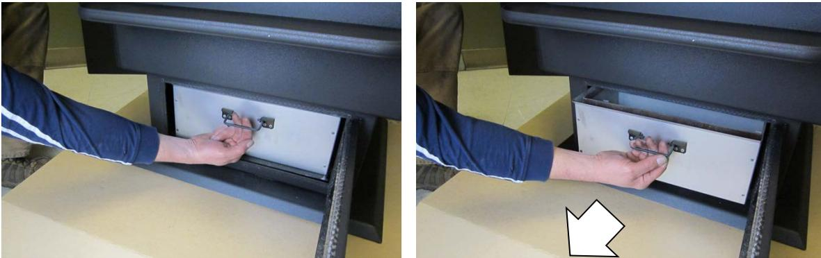
3. Remove the ashpan from the appliance and properly dispose of the ashes (see “Disposal of Ashes” on page 32 for details). You may wish to clean the area below the firebox.
